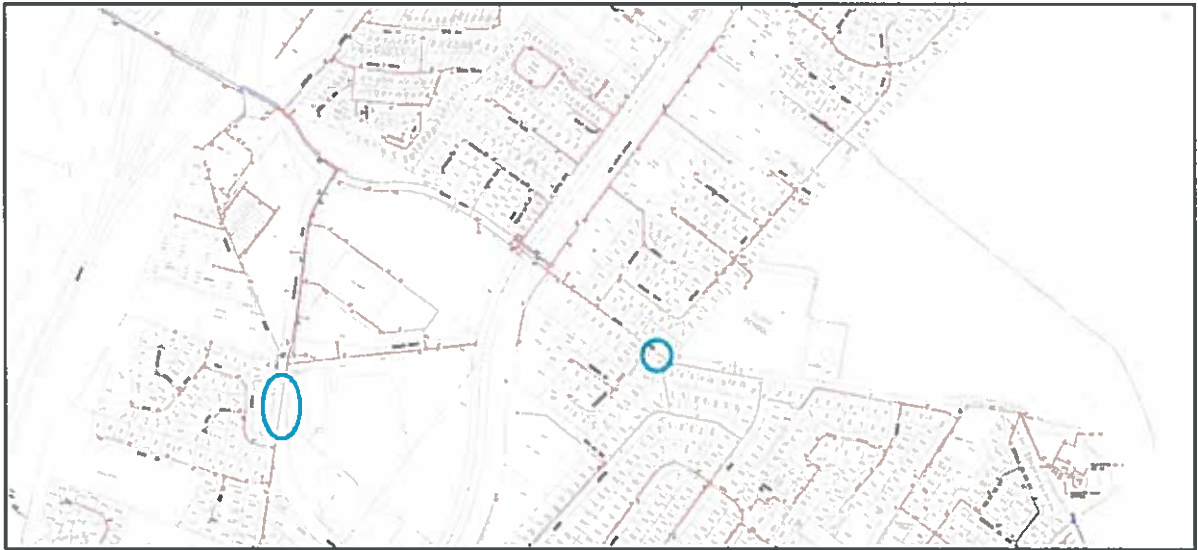
Figure 2 - System Bottlenecks (8" Pipes, circled in blue)
